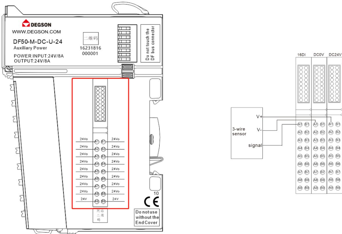
Each of the 16 channels can provide a rated voltage of 24VDC for external loads.
